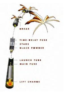
**Figure 3-1: Display Firework Schematic** (from <u>www.pbs.org/wgbh/nova/fireworks/anat\_flash.html</u>)
